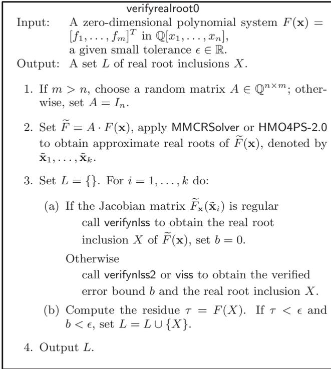
**Figure 1: The Verification Algorithm for Zero-Dimensional Polynomial Systems.**
