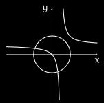
Example: The polynomials  $p_1 = x^2 + y^2 - 4$  and  $p_2 = (x-1)(y-1) - 1$  induce a decomposition of  $\mathbb{R}^2$  into 13 cells:
